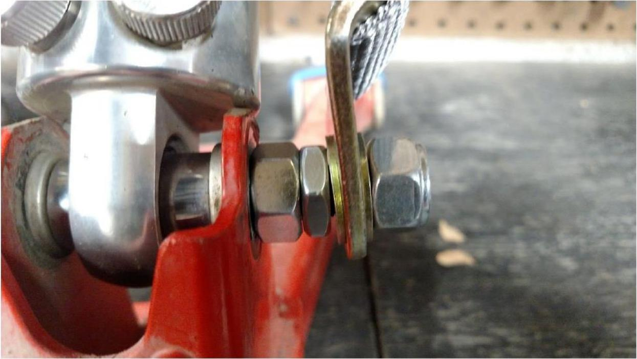
Show above is the correct limiter strap orientation for most applications.
